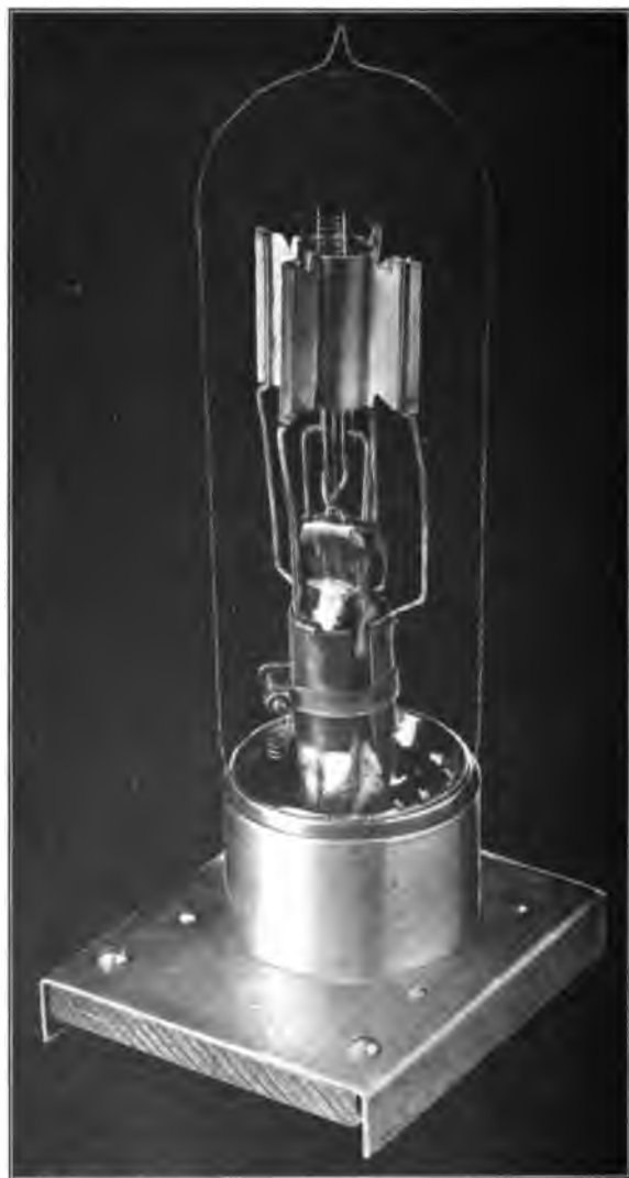
Plate 4. —Three-electrode vacuum tube used as high power oscillator and modulator. The plate has been forced downward to expose the grid and filament axially mounted. Note the cooling flanges on the plate. Signal Corps tube type VT-18.
